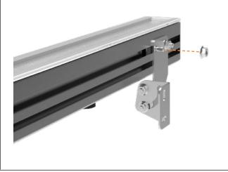
Step 3 HINT: Tightening and loosening the nuts on the mounting studs will allow the bracket to slide within the rail. This can be useful in shifting the luminaire a small amount, even after installation. Repeat these steps for each bracket on each luminaire.
