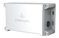
The PowerSync™ Data Injector combines the convenience of standard wiring methods to translate control signals into a digital format that can be transmitted over standard copper wire. This allows highly granular addressing and high speed digital control of every luminaire, using only four wires. The PowerSync™ Data Injector accepts a growing list of standard protocols (0-10 V, DMX/RDM), for simple integration with a wide selection of control systems using these industry standard protocols.
