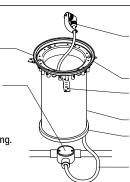
Waterproof quick connector, Submersible plug and cable. Ensure free cable reaches beyond height of collar for luminaire connection.
