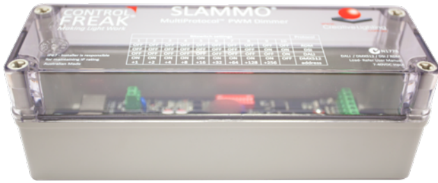
PCB in IP67 enclosure with optically clear lid
