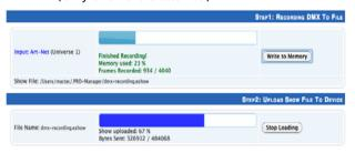
After selecting the options, you can select the input (Art-Net and universe or DMX) and click on "Record DMX" to start the recording. The recording is saved onto a file, and is only transferred to the PRO Mk2 memory when recording is stopped using the "Stop Recording" button.
